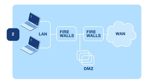
In this case, the two firewalls have to be configured perfectly to allow traffic through. And if you follow the industry standard of having firewalls from different providers, it doubles the chance for a misconfiguration to occur, making access difficult for legitimate users.
