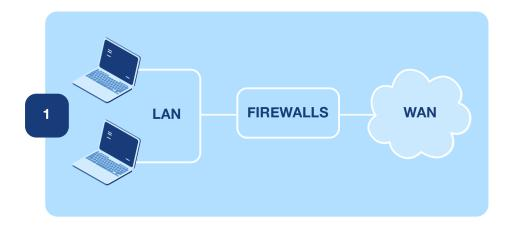
From this, we can see that the system has security added on, in the form of a firewall. In this case, the security is only as good as the configuration of the firewall.
